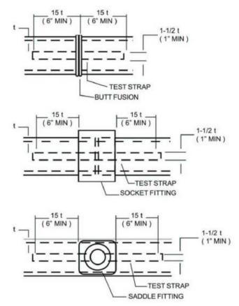
Figure 1 ASTM F2620 Specimens for bent strap tests
