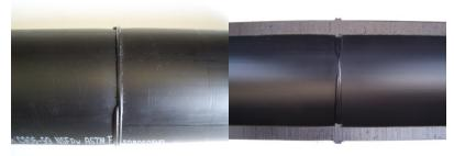
Figure 8 - Incomplete facing or insufficient heat time
