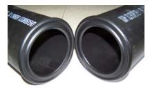
Figure 2 - Unacceptable Concave Melt Appearance
