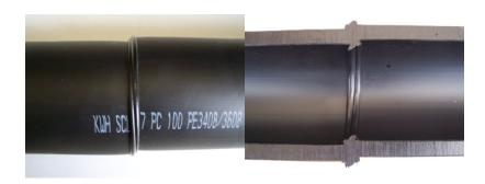
**Figure 7** - Pipe misalignment (high-low misalignment)
