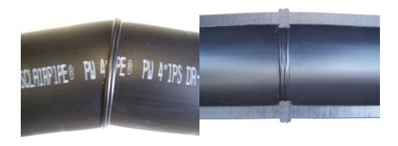
Figure 9 - Field mitered joint( pipe angled in the fusing unit)
